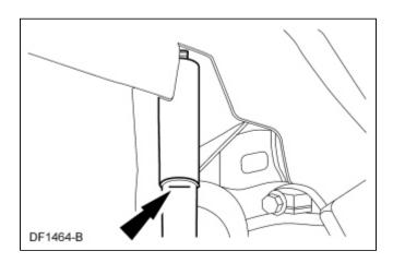
5. Using 2 screwdrivers inserted through the access hole, depress the tabs of the panhard rod bolt cover retaining clip and remove the cover.
